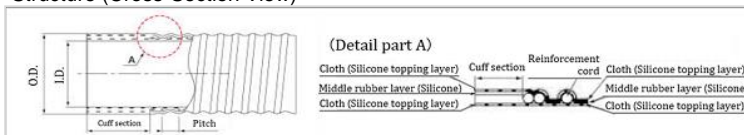
Structure (Cross-Section View)
