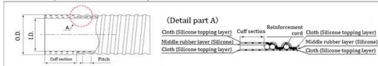
Structure (Cross-Section View)
